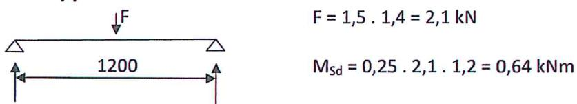
Pásek P10x60 - A =  $600 \text{ mm}^2$ ; J<sub>y</sub> =  $0,180 \cdot 10^6 \text{ mm}^4$ ; W<sub>y</sub> =  $6,00 \cdot 10^3 \text{ mm}^3$ ;
